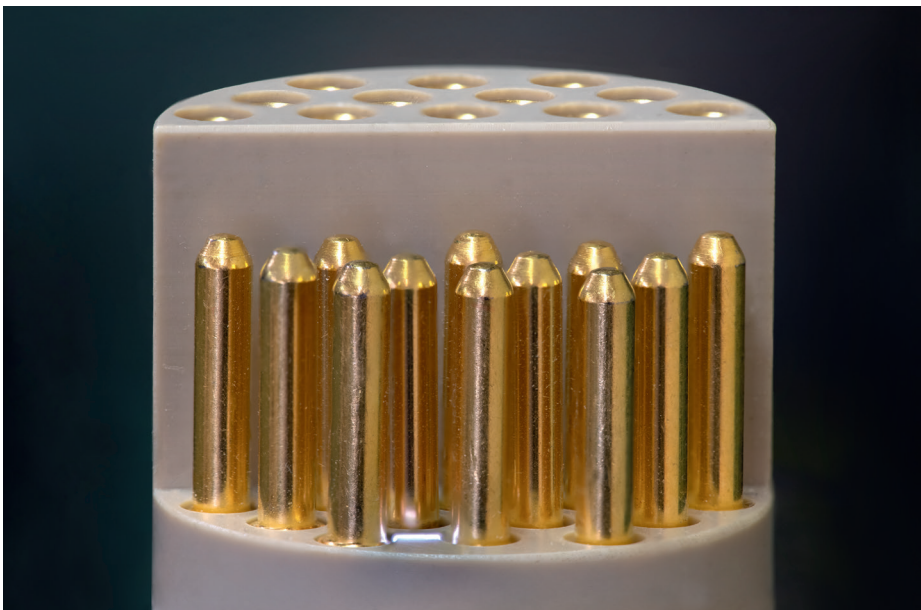
Figure 5 Corona effect visible between two electrical contacts at the surface of the connector insulator
